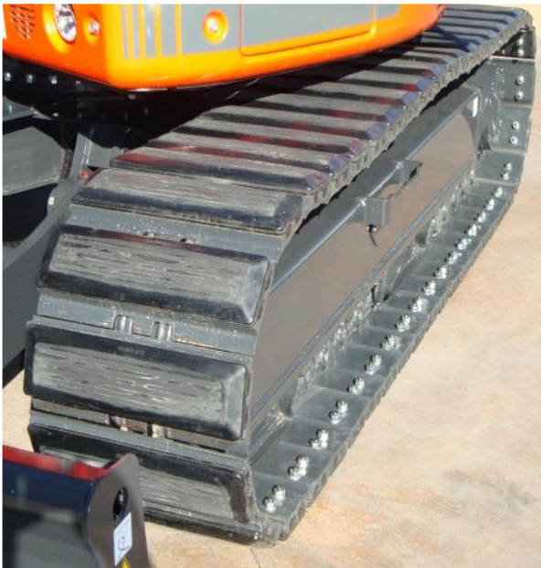
8-hole steel tracks with screwed-on rubber pads Bolton
