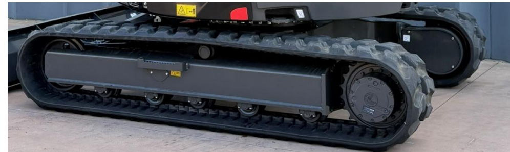
Rubber tracks – with continuous track guide and a profile that always runs to the center of the track – a good standard even in the 10-ton range
