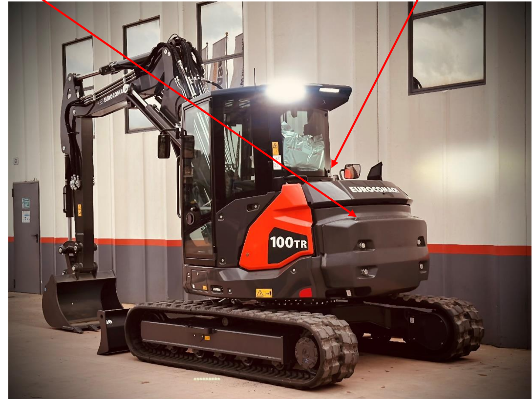
Additional rear ballast of 440 kg is installed inside the backpack (standard on 100 TR)
