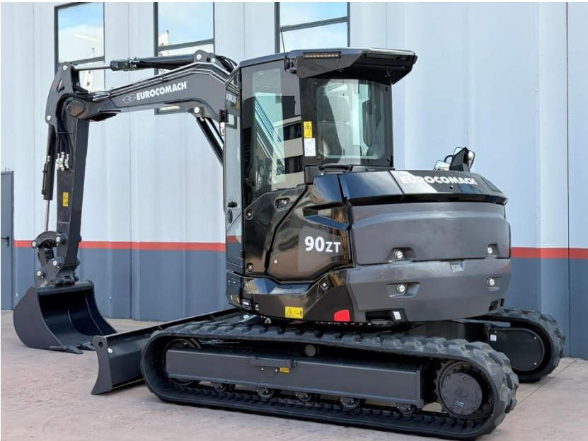
Rubber tracks – with continuous track guide and a profile that always runs to the center of the track – a good standard even in the 10-ton range
