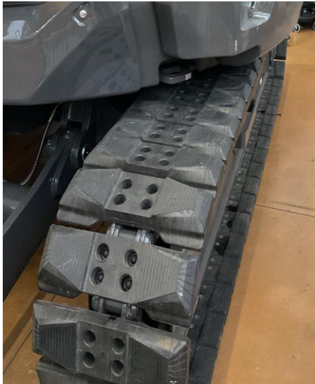
GEOGRIP BRIDGESSTONE (vulcanized iron chains screwed directly onto the ground)
