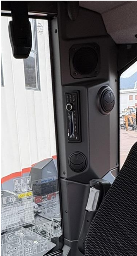
Sun blind, coat hooks, interior lighting, Bluetooth radio with hands-free system (opt. DAB+) and several ventilation units
