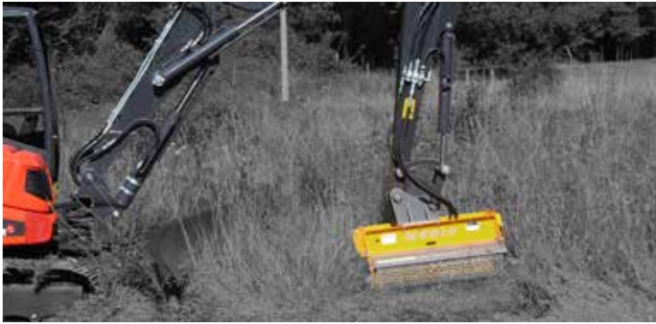
Single/double effect hydraulic system with electrical containment (70 lt/min)
