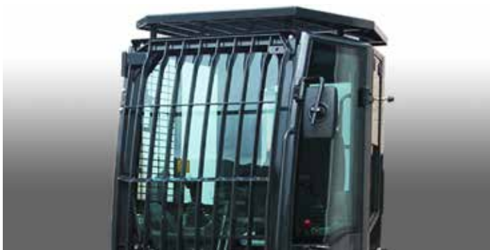
Additional front and rear protective grills with FOPS level II certification
